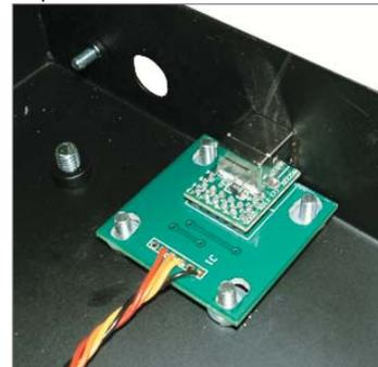
Insert USB into aperture, insert fixings and tighten.
