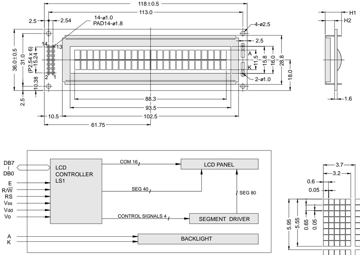
The tolerance unless classified  $\pm 0.3\text{mm}$
