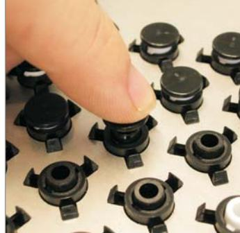
Flip key chassis over and install key plugs to all the keys.
