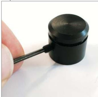
Partially install grub screw into both knobs using allen key
