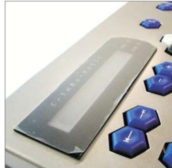
Align the display cover with the LEDs and apply even pressure.
