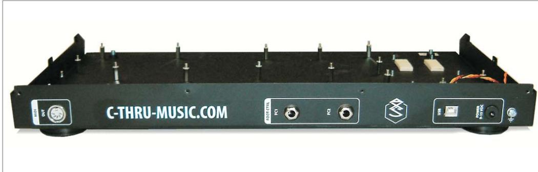
Remove nut from connector, insert body through hole, replace nut and tighten.
