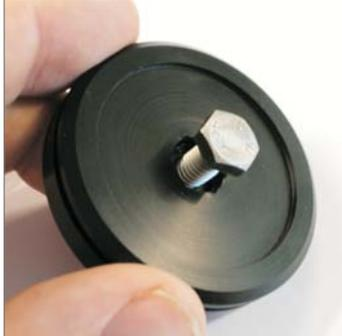
Push M6 fixing into foot until head is level with surface.
