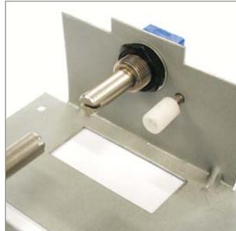
Install a M3 x 6 screw through the chassis and insert a spring stop.
