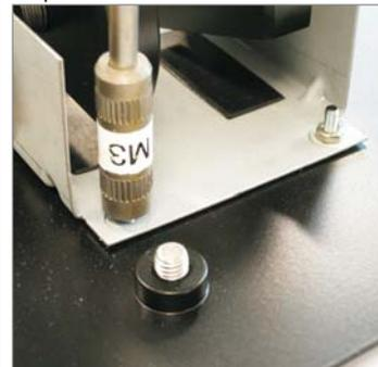
Apply a M3 nuts and shakeproof washers to each stud and tighten.
