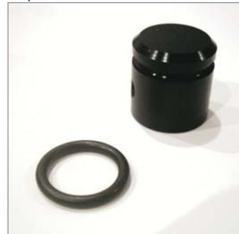
Roll rubber O-ring down knob into recess.
