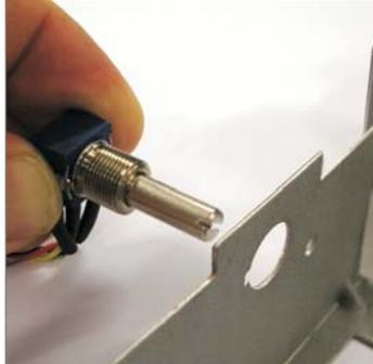
Load pot ensuring location lug lines up with keyway in the wheel chassis
