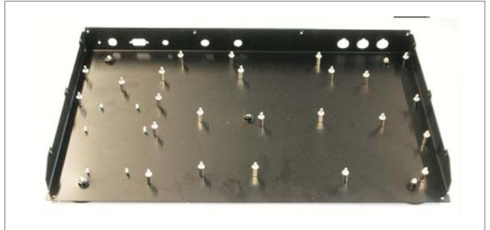
**N.B.** Take care not to shear threads by over tightening standoffs.
