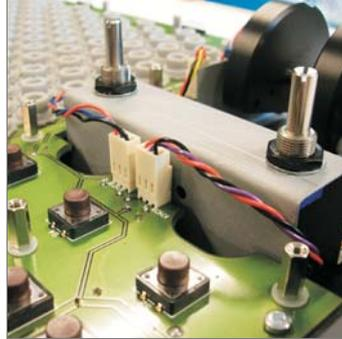
Insert knob pots connectors onto PCB
