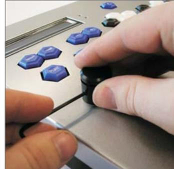
Tighten grub screws using a 2mm allen key
