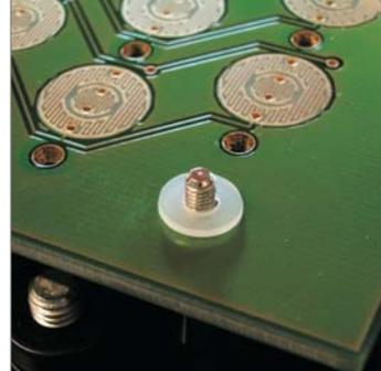
Install nylon washers, excluding the four standoffs in center of the board
