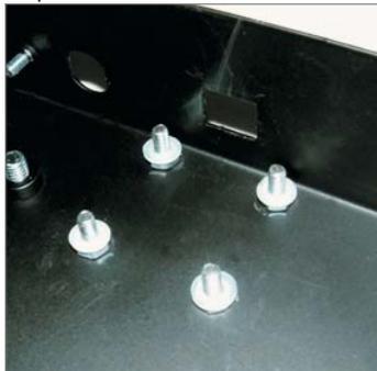
Insert M3 nut and nylon washer onto each of the USB mounting studs.
