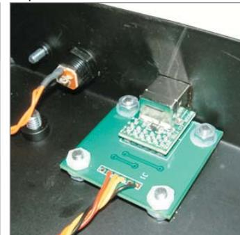
Remove nut, insert power connector, replace nut and tighten.
